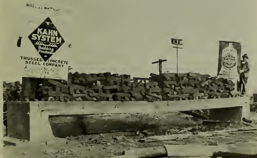
Load 51,000 lbs.; 370 lbs. per sq. ft. Deflection 1.50 in. Designed for 10,240 lbs. (75 lbs. per sq. ft.)
