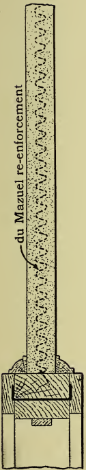
PLAN OF SINGLE PARTITION OR WALL SHOWING MEANS OF CONNECTION TO WINDOW OR DOOR FRAME
