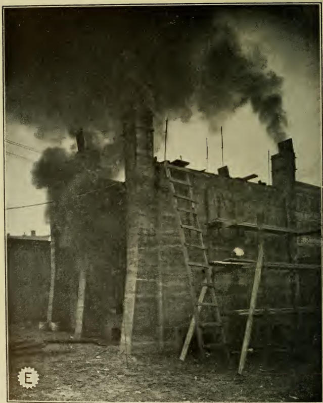
An oak fire was started and kept up for four hours, so as to give a uniform heat throughout that time of from 1,750 to 1,860 degrees Fahrenheit.
