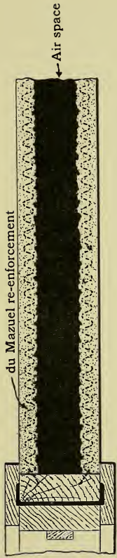
PLAN OF DOUBLE PARTITION OR WALL SHOWING MEANS OF CONNECTION TO WINDOW OR DOOR FRAME
