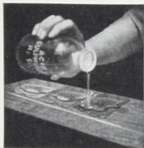
The above experiment consists of pouring sulphuric acid on COLORFLEX which has been placed in a single coat only on a board. Sulphuric acid does not even affect the gloss.
