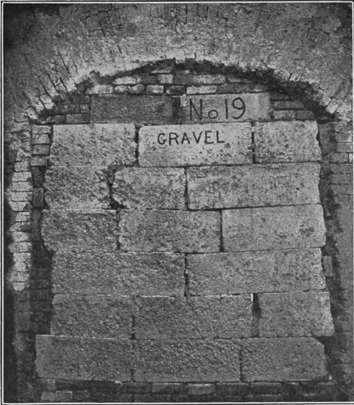
Fig. 116. Appearance After Test of Panel Containing Gravel-Concrete Beams
