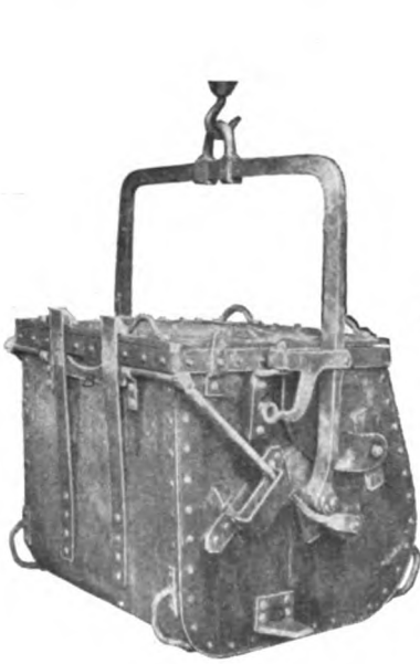
Fig. 27.—Cyclopean Bucket for Depositing Concrete Under Water (Closed Position).
