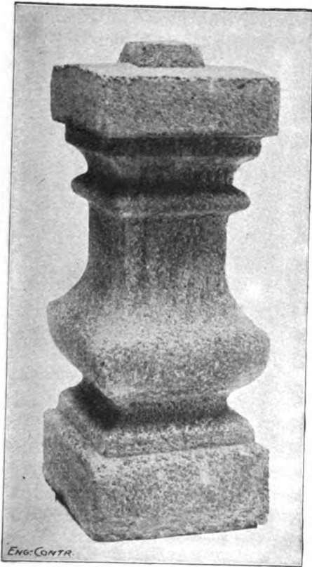
Fig. 47.—Concrete Baluster Finished by Scrubbing and Washing.
