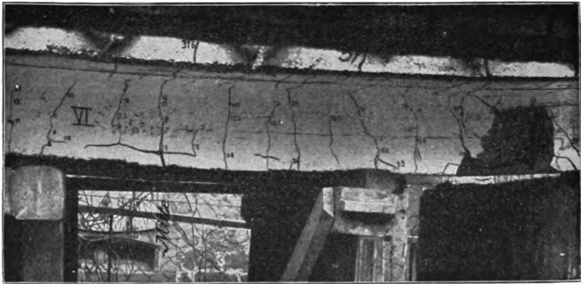
FIG. 150.—Beam VI, under the breaking load.
