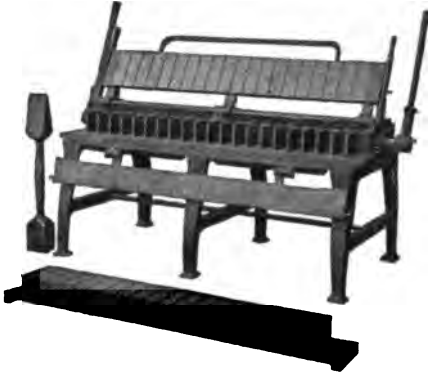
FIG. 18.—South Bend 20-Brick Machine.
