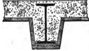
FIG. 101.—Encasing the Bottom Flanges with Lathing.
