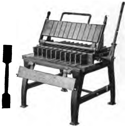
FIG. 19.—South Bend 10-Brick Machine.
