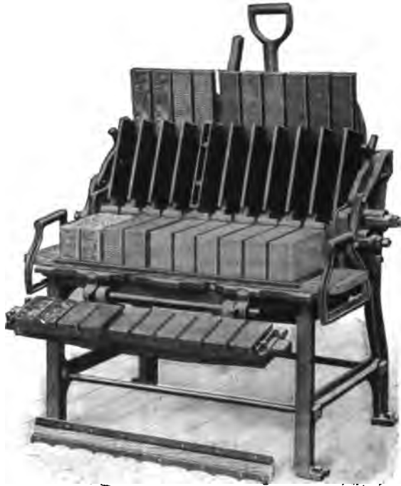
FIG. 22.—Cement Machinery Company—10-Brick Machine.
