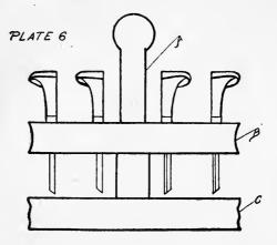
and eight inches in diameter; base C is same size. In all there will be three pieces. There can be two rows, holding fifteen to twenty gravers. This stand, placed on a table, the engraver can turn it around and readily select the graver wanted, and by keeping them in this stand they are free from any danger of point being damaged. The piece B turns on shoulder of center piece A.
