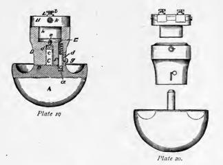
adjusted as desired. The head turns on a pivot extending up through the base; the same is adjusted at any height by a key which operates on a set screw holding said pivot firmly at height desired.
