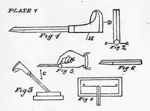
After breaking the graver off the desired length and grinding or whetting the end to an angle of 45 degrees, we then grind the under sides E, Fig 2, back about half an inch and on an angle as shown at Fig. 6.
