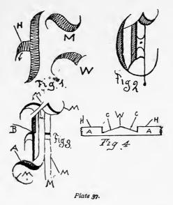
dicular bar we can, by holding the cutting edge of the flat tool on a slight angle begin the bar quite pointed, in so doing soon as we have rolled the graver two or three times to effect the wriggle we turn the tool so the cutting edge is horizontal with the bar and so continue until we near the end, where, if desirous of making same pointed, we proceed as in the beginning by turning graver
