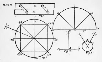
It has been my experience in instructing students that many fall short of the exact conception of an angle of 45 degrees, without the aid of an angular circle of a protractor. A protractor is a half circle and a complete circle consisting of 360 degrees, a protractor would therefore consist of 180 degrees.
