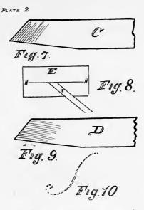
to make two, as with the second we can finish the first, and it requires a very little more time to make two), get a piece of hard wood four inches long and one inch square, finished flat on all sides; now take a piece of 0000 emery paper (which you can get at any material house), coat the back or paper side with mucilage, treating one side of the block in the same manner. Allow it to stand two or three minutes, then place the paper on
