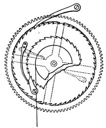
Fig. 181.—Maintaining power for weight clock.
