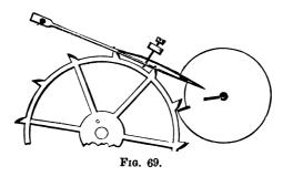
the wheel to unlock, the sunk part of the body of the wheel allowing the locking stone to pass.
