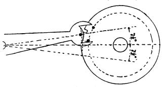
Fig. 166.—Savage's two-pin escapement.
