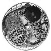
Fig. 21.—Watch movement with "stackfreed."
