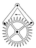
Fig. 155.—Pin pallet escapement.
