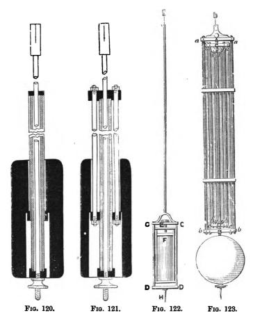
corresponding internal thread, and was screwed on to the zinc tube, so that the acting length of zinc tube could be adjusted by screwing the collar on or off. This seems a more rational way of proceeding.
