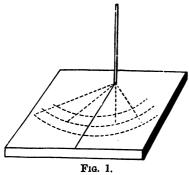
circles, a quarter of an inch from one another, on a flat stone, and let the outmost circle be but little less than the stone will contain. a pin perpendicularly in the centre, and of such a length that its whole shadow may fall within the innermost circle for at least four hours in the middle of the day. The pin ought to be about an eighth
