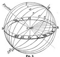
the hour spaces cannot be equal. A sun-dial may be regarded as a circle round the earth, or as the edge of a disc which passes through the centre of the earth from the spot where the dial is fixed. a, b, c, d, e, f, g, etc., are longitudinal circles, representing the hours, B the spot where the dial is situated, D the
