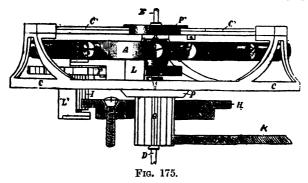
is concerned, may be regarded as a circular rack. The lower pivot, D, of the carriage runs in the main plate of the movement, and carries the seconds hand; the upper pivot, E, rotates in a high and long bridge which spans the carriage. LL are the cocks for escape pinion pivots.
