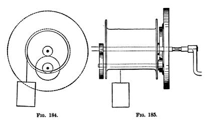
the winding is completed. During the going of the clock the whole system turns with the barrel arbor, so that there is no extra friction from the maintaining work. It is not absolutely necessary to have both of the wheels which run on study at the end of the barrel, and sometimes one of them is omitted.
