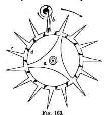
a, escape wheel; b, impulse pallet; c, locking teeth; d, impulse teeth; c, ruby roller.
