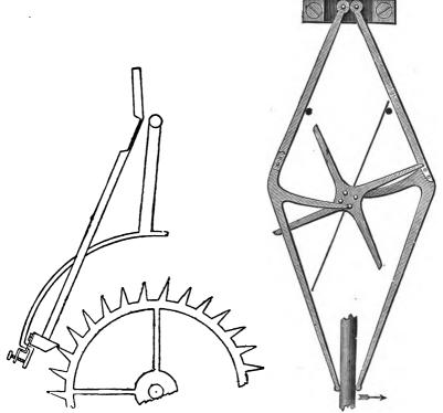
Fig. 158.—Reid's gravity escapement.
