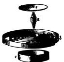
Fig. 20.—Mainspring and barrel.
