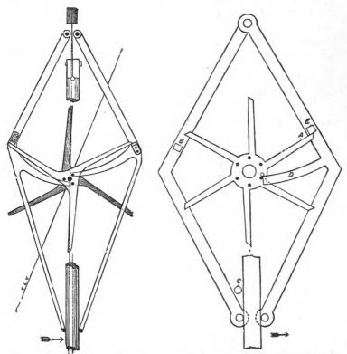
Fig. 156.—Double three-legged gravity escapement.
