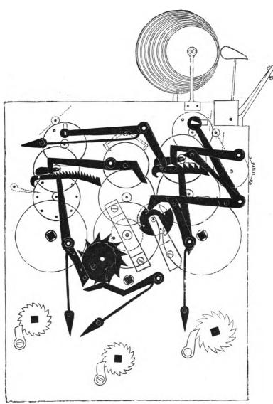
Fig. 126.—Striking mechanism of quarter-chime clock.
