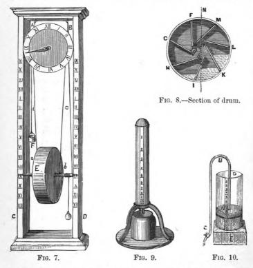
It has seven water-tight metallic partitions, F f, G g, H h, I i, K k, L l, and M m. If, now, the cord be wound around the axis until the drum rises to the top of the frame, and the drum be left to obey the force of gravity, it will of course tend to fall, and the cord resisting this tendency will cause it to revolve rapidly as it descends. But if we introduce water into the vessel, it will be
