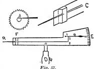
at 1; 2 and 2 are pivot joints only, and do not go through the body; fig. C will perhaps give a better idea of the end R. To center with this tool, unscrew your rest and remove it, then place the shaft C, fig. 57, in rest holder and adjust it till the needle point R touches the top of hole as
