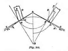
not thoroughly comprehend, and we would advise a close study of Fig. 203, which will make it perfectly clear, as we show both a wide and a narrow pallet. GH represents the primitive, which, in this figure is also the real diameter of the escape wheel. In measuring the lifting angles for the pallets, our starting point is always from the tangents
