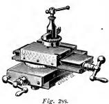
lathe; it is so universally used by all watchmakers that a full description is superfluous. Fig. 288 is a Waltham, and is a fair example of a modern slide rest for watchmakers' use. The tool holder varies with the different makers, but the rests proper are all made on the same general principle: that of two sliding beds working at right angles to one another and carrying a tool holder, which is capable of being raised or low-
