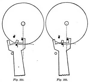
When treating on the width of the ruby pin, we mentioned the Savage pin roller escapement, which we illustrate in Figs. 221 and 222. This ingenious arrangement was designed with the view of combining the advantages of both wide and narrow pins and at the same time without any of their disadvantages.
