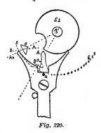
in case the guard point at that moment be thrown against the roller. We will now examine the question from the standpoint of the double roller; S2, Fig. 220, is the safety roller; the corner of the crescent has
