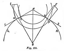
as the lever arms AMO and ANP, Fig. 108, are equal lengths. It will be noticed by examining the diagram, that the pallets are bisected by the 30° lines EB and FB, one half their width being placed on each side of these lines. In this pallet we have two locking circles, MP, for the engaging pallet, and NO for the
