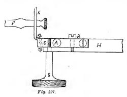
we require a little tool of which we show a plan in Fig. 227, and a side view in Fig. 228. His a piece of steel of the form of the shank of the slide rest cutter. D. Fig. 228, is a steel table pivoted on it, by the shoulder screw S. C is a heavy spring screwed to the table D. A is a set screw for deflecting
