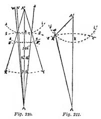
Fig. 210 than in Fig. 211. The action in the latter begins much further from the line of centers than in the former and outlines an action which should not be made.
