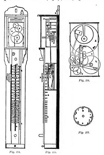
wheels, ending with a lone pinion. The first wheel, a, carries pins which control the hammer to strike the gong T; the second wheel, c, carries an elbow which stops the train and raises the bascule L with one end, while
