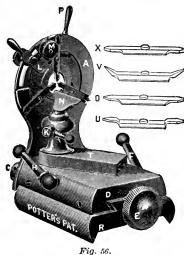
bed and fasten it there; after which move the sliding jaws inward until they bind lightly on the bit of straight wire held in your chuck, and in this position again tighten the nuts C C. Once adjusted to accurate center in this way no further adjustment, whatever the size of work to be operated upon, is required, until another change of jaws.
