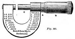
Watchmakers will especially appreciate micrometers of this form. This tool will be found very useful for gauging mainsprings, pinions, etc. In the caliper, shown by cut, the gauge or measuring screw is cut on the concealed part of the spindle C, and moves in the thread tapped in the hub A; the hollow sleeve or thimble D is attached to the spindle C and covers and protects the gauge screw. By turning the thimble, the screw is drawn back and the caliper opened.
