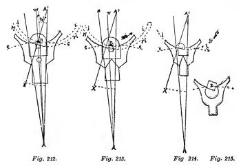
hand the widest ruby pin for which there is any occasion is one beginning the unlocking action on the line of centers, Fig. 212; this entails a width of slot equal to the angular motion of the fork. We see here the advantage of a wide ruby pin over a narrow one in the unlocking action. Let us now examine the question from the standpoint of impulse action.
