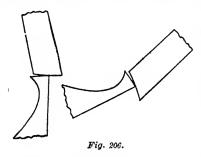
latter part of the lift the action becomes quicker on the disengaging pallet and slower on the engaging.
