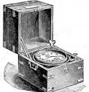
CHRONOMETER. A portable time piece of superior construction, with heavy compensation balance, and usually beating half seconds; intended for keeping very accurate time for astronomers, watchmakers, etc. See Fig. 6o.
