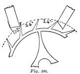
val of 24 degrees from tooth to tooth, which is also the angle at which the locking faces of the teeth are inclined from the center, which fact will be found convenient when we come to cut our wheel.
