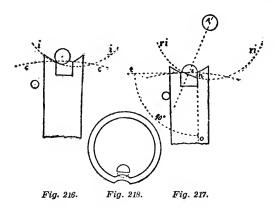
width of the pin, and plant the center x on the line n t. We can have the center of the pin slightly below this line, but in no case above it; but if we put it below, the pin will be thinner and therefore more easily broken.
