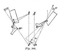
and NN2, representing the paths of the pallets. It will be noticed that UNF and TNB are opposite and equal angles of 12°. For practical reasons, from a manufacturing standpoint, the angle on the tooth is made just twice the amount, namely 24°; we could make it a little less or a little more. If we made it less than 20° too great a surface would be in contact with the jewel, involving
