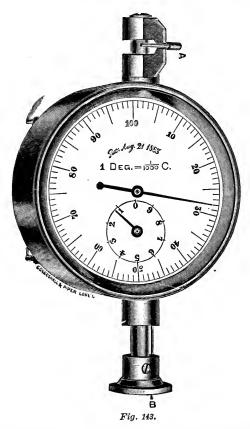
Fig. 143 shows the piece of work marked A, being gauged, while B represents a stationary spindle to get the depth of a hole or recess or the thickness of any piece of work which will be indicated on the dial.
