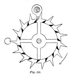
the circle of the escape wheel and the duplex roller intersect each other sufficiently that the escape teeth cannot pass except when the tooth drops into the notch of the roller and is traveling in the same direction of the escape wheel. At the instant that the tooth passes
