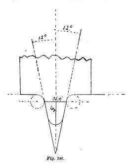
concave. Then cut ten teeth on it and harden and temper, after which it is ready to be used in a wire chuck in the head stock of the lathe.
