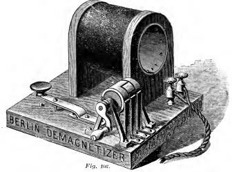
or three feet. Keep turning commutator at regular speed. Release key before ceasing to turn. It is not necessary to remove the movement from the case nor to let it remain in the magnet. While the current is on and the handle being turned with key down, insert the watch into the opening and proceed as above.
