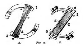
96 the flat rim is made of brass, the arm A of aluminum, the compensating arm Z is of zinc. The balance rim is united to the arm at a either by rivets or pivots, similar rivets b b form the connection for the compensating arm; they are placed quite close to a a. In heat the zinc arm Z will expand much more than the aluminum arm A, and cause the rim to move inwardly, as indicated by the dotted line. Both arms, A and Z in this case of are equal length; the regulation
