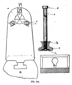
points in which it differs from that employed by the machinist is the shape of the jaws and the mode of fastening to the lathe bed. a shows the rest in position on the lathe bed, looking from right hand end of
