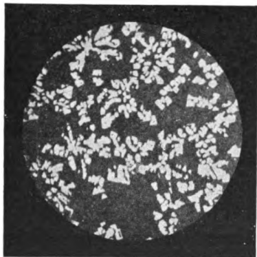
FIG. 73.—Pb-PbS Alloy, 18.7 Per Cent PbS; PbS Light, Metal Dark (Friedrich and Leroux).
