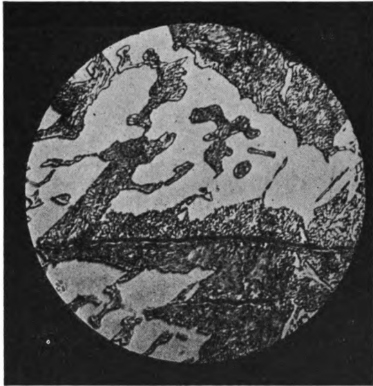
FIG. 60.—Graphite in Eutectic, Strongly Enlarged (Goerens).
