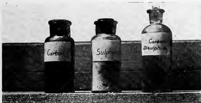
FIG. 5.—The black solid, carbon, combined with the yellow solid, sulphur, forms the colorless liquid carbon disulphide.
