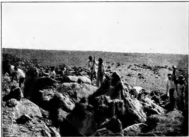
FIG. 46.—Opening up a trench after blasting; extraction of caliche by piece work.
