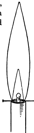
FIG. 104. A match head suspended in lower part of gas flame is not ignited
