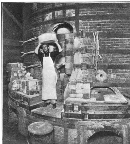
FIG. 163. The manufacture of pottery; burning the ware in a kiln
