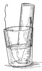
F1G, 3.—Apparatus used in preparing nitrogen.
