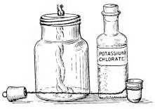
FIG. 2.—Apparatus used in preparing oxygen.
