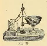
other end is then hermetically sealed at the blast-lamp. The branch containing the crystals is then heated in a water-bath, while the other branch is cooled in a freezing mixture (Fig. 39). The hydrate of chlorine breaks up into water and chlorine, and the greater part of the latter is disengaged, and condenses by its own pressure into a deep-yellow liquid, which collects in the cooler limb of the tube (Faraday).
