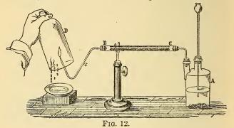
duced. The hydrogen evolved is made to traverse the tube CB, which is filled with fragments of chloride of calcium; after having been dried by this substance, which is very avid of
