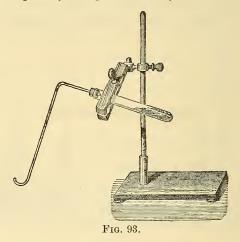
coal by heating the mixture in a glass tube by the aid of a spirit-lamp (Fig. 93). Carbon dioxide is disengaged.
