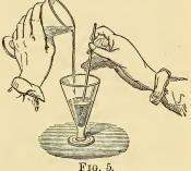
substance possesses a strong, lye-like, alkaline taste, very easy to distinguish from that of the acid. The color of the blue litmus is not affected by this liquid, but if a few drops of the litmus solution, previously reddened by an acid, be added, the blue color is immediately restored. This caustic substance has properties which are different from those of acids, and which are called basic or alkaline properties. Potassium hydrate is an alkali or powerful base.
