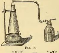
holders of laboratories, etc., a mixture of potassium chlorate and manganese dioxide is heated in a sheet-iron or copper retort (Fig. 18).
