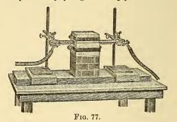
recently supplanted by a device known as the electric furnace, in which the energy of powerful electric currents is converted into heat. The temperatures which can be thus reached and maintained far exceed 3000°. Nearly all those bodies which were formerly regarded infusible and non-volatile have been melted and vaporized in the electric furnace, and many new products have been obtained by its means.
