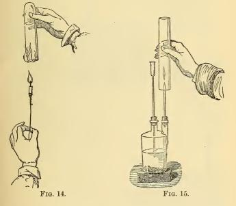
rapidly and at regular intervals. These conditions are realized by burning a small jet of hydrogen in a somewhat large tube (Fig. 15). The flame is drawn away from the jet by the draft in the tube, but immediately recedes as the ascending hydrogen gas mixes with the air, at the same time producing a faint explosion, and the rapid succession of these explosions produces a musical tone.
