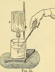
56). When the experiment has terminated, the volume of gas will be found to have doubled. 200 volumes of oxygen are added to the 400 volumes of gas thus obtained, and a spark is passed; an explosion takes place, and after making the
