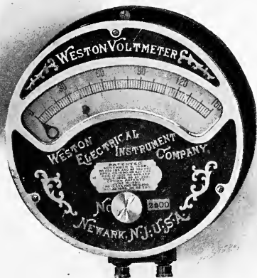
Fig. 7—Voltmeter used in Electro-plating Manufactured by Weston Electric Company, Newark, N. J.
