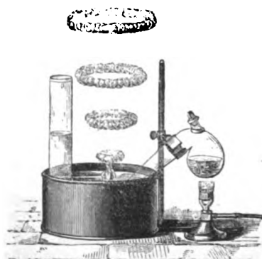
Fig. 209.—Preparation of phosphuretted hydrogen.
