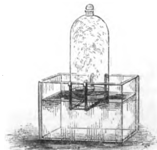
Fig. 120.—Preparation of nitrogen.
