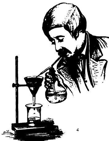
Fig. 115.—Washing a precipitate.
