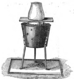
Fig. 210.—Extraction of arsenic.
