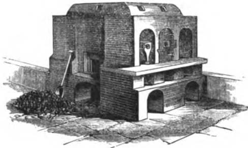
Fig. 228.—Silesian zinc furnace.
