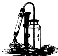
Fig. 146.—Preparation of nitric peroxide.
