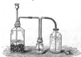
Fig. 186.—Preparation of hydrosulphuric acid.
