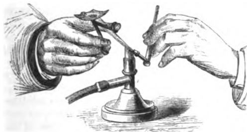
Fig. 112.—Fusion of platinum foil.
