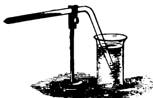
Fig. 129.—Liquefaction of ammonia.
