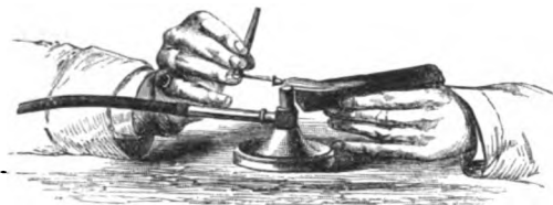
Fig. 107.—Reduction of metals on charcoal.
