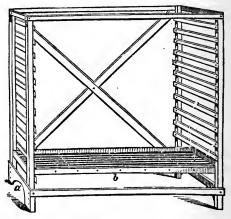
(b) is a rack four feet long and about one and one-half feet wide, made of common wall lath nailed together one-tenth to one-fourth of an inch apart, according to the size of the fruit to be dried. A lath or strip of board one inch wide is nailed round the edge to prevent the fruit's falling off. The whole expense is but a mere trifle. Any person who can drive nails can make it. If laths are not to be had, strips of boards will do as well.
