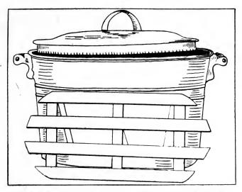
Fig. 1. A false bottom of wood (or of wire) placed in an ordinary wash-boller makes a good outfit. Note rim on cover.
