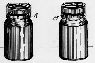
FIG. 17. Positions of Clamp on Glass Top Jar before and after Sterilizing. A. Before and during sterilization. B. After sterilization.
