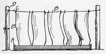
FIG. 29. Apparatus for Sun Evaporation of Fruit Juices. A. Shallow trough or pan to hold juice. B. Pieces of cheesecloth for evaporation of juice. C. Line to hold cloths. D. Posts for support of line.
