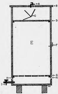
FIG. 50. Plan for Upright Vinegar Generator for Farm Use. A. Delivery pipe ings. Corn cobs, or for fermented juice. B. Cover. C. rattan shavings may Tilting trough to distribute liquid over false head. D. Perforated false head. E. Main cylinder of generator coal or coke in large filled with shavings. F. Thermome- pieces may be used for ter. G. Walls of generator. H. Air distilled alcoholic liqinlets. I. Outlet for vinegar.
