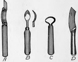
FIG. 2. Types of Knives for Preparation of Fruit. A. Pomona peeling knife with guard to regulate thickness of peelings. B. Peach pitting spoon. C. Pear coring knife. D. Fruit cutting knife.
