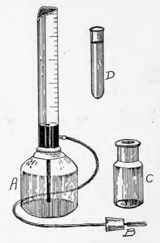
FIG. 51. Leo Acid Tester for Testing Strength of Vinegar. A. Water reservoir and graduated cylinder. B. Measuring spoon for baking soda. C. Bottle in which vinegar and soda are mixed. D. Tube for measuring vinegar.
