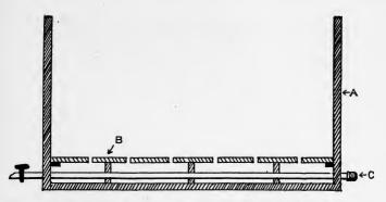
FIG. 26. Wooden Vat with Steam Coil for Use in Sterilizing Bottles of Juice or Cans of Food. A. Walls (of wood). B. False Bottom. C. Steam Coil.
