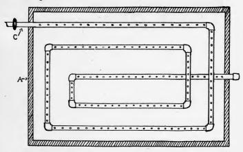
FIG. 27. Plan for Arrangement of Steam Coil of Fig. 26. Showing perforations for escape of steam for direct heating of water.
