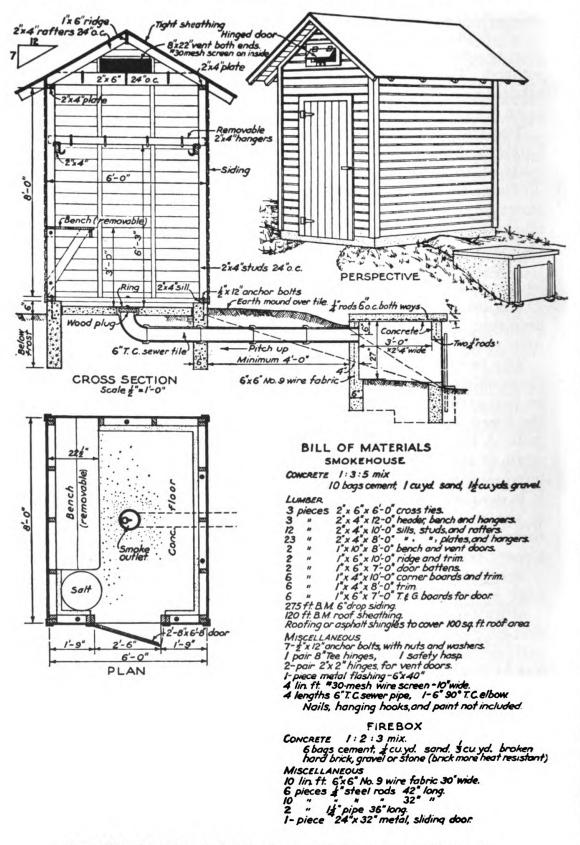
FIG. 195A. Drawing and bill of material for frame smokehouse.
