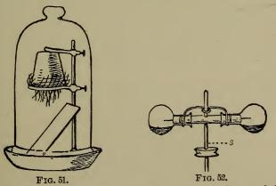
FIG. 51.—Inverted flower-pot under a bell-jar. One tenth natural size. FIG. 52.—Rotating apparatus. s, steel rod bearing a pulley by means of which it is rotated. One fifth natural size.
