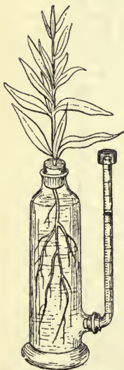
Fig. 43.—Apparatus for estimating the Absorption of Water by the Roots, and the Loss by Transpiration from the Leaves.
