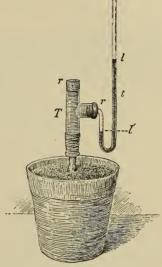
FIG. 25. — Apparatus to Measure Root-Pressure.
