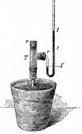
FIG. 23. Apparatus to measure Sap-Pressure.
