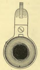
FIG. 29.—Illustrating the rifling used in our Springfield model 1906,—four lands and four grooves. The grooves are only four one-thousandths of an inch in depth, five to ten times less than those used in old-style barrels, intended for bullets of pure lead. The caliber of the bullet of course must be large enough to fill the grooves on each side; the Springfield bullet is therefore .308 caliber, while the barrel before rifling is .30 caliber.
