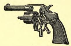
FIG. 49.—A LATER TYPE OF COLT REVOLVER Showing cylinder hinged to fall to one side for easy extraction of shells and reloading.
