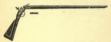
FIG. 32.—Breechloader of date about 1700, handed down as a relic of Philip V, King of Spain. The iron cartridge it used is shown; a hole in its wall near the base admitted the igniting fire from the snaphance igniter.
