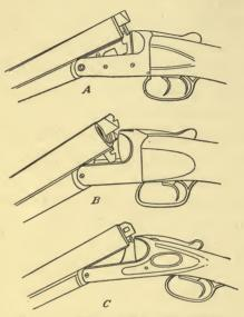
FIG. 79.-.-TYPES OF SHOTGUN BOLTS
