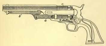
FIG. 50.—COLT'S REVOLVER, WITH JOINTED RAMBOD
