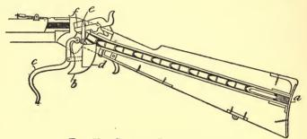
FIG. 51.—SPENCER REPEATING RIFLE a, follower; b, carrier block; c, lever guard; d, breech block; e, extractor; f, guide.
