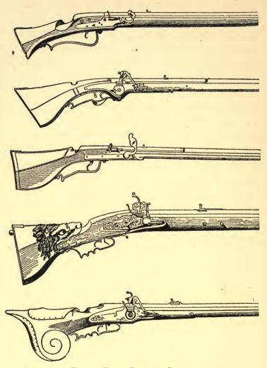
FIG. 6.—EARLY TYPES OF STOCKS Used on arquebus and musket. They include both wheel-lock and snaphance igniters.
