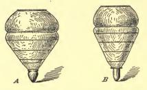
FIG. 54.—Of these two tops, A and B, the former is the thicker of the two. If both be spun at the same speed, A will stand up longer than B. Similarly the bullet with the greater diameter will remain point foremost longer than the thinner and when both are rotating at the same speed, length and material being alike.
