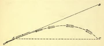
FIG. 58.—Arrows indicate the changing directions from which air pressure comes against the bullet.
