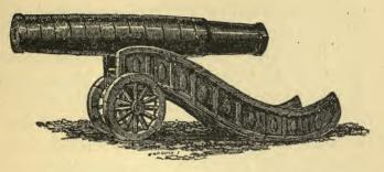
FIG. 1.—THE "MONS MEG" (Edinburgh Castle) Made about the middle of the 15th century, this huge iron gun remains to us a most interesting relic. Its bore is 20 inches, though the powder chamber is of less diameter to decrease the bursting effect of its charge. It fired balls of stone weighing about 300 pounds.
