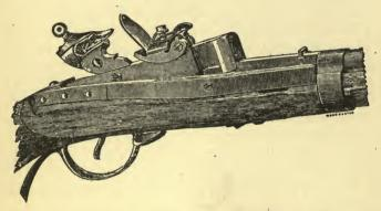
FIG. 34.—HALL'S AMERICAN BREECH-LOADING RIFLE This was the first successful breechloader, a remarkable gun in its time. The combustion chamber was a movable part which tilted upward for loading and was then depressed for firing. The flint-lock igniter was affixed to the tilting chamber.
