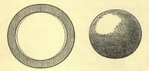
FIG. 27.—BULLET AND MUZZLE OF THE LANCASTER RIFLE The oval shape of the barrel progressed spirally from breech to muzzle and the oval-shaped projectile in following this twisting path was caused to rotate. Fouling of the barrel quickly made loading difficult, while the odd-shaped bullet did not fly as accurately as the true sphere.
