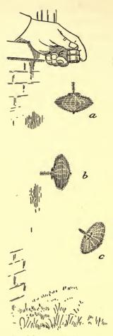
FIG. 22.—Experiment with a spinning top, showing how the spinning body tends to maintain the position assumed when released. It must be remembered that this is only a tendency, which can be overcome when any force or obstacle of sufficient power intervenes. A new position thus given will then be maintained until some exterior influence again interferes.
