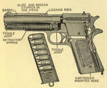
FIG. 84.—COLT AUTOMATIC PISTOL, GOVERNMENT MODEL (Browning Pistol) Sectional view, showing mechanism.
