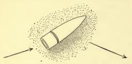
FIG. 63.—In seeking the cause of the disturbance called drift, which carries the rifle bullet to right or left, according to its rotation, some authorities assert that the air buoying the missile from below causes a rolling action, much like that which takes place when a rotating body is dropped on the floor. The picture illustrates this theory.
