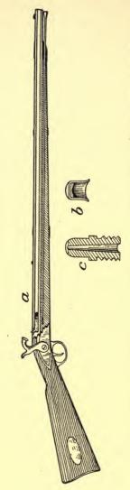
FIG. 9.—a, The type of musket in common use by soldiers from 1830 to 1860; b shows a cross-section of Shaw's percussion cap, first made of steel and then of copper; c is a cross-section of Shaw's nipple upon which the cup was exploded and through which the igniting flame was led into the charge in the breech of the barrel.
