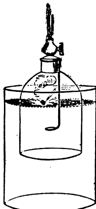
Fig. 20. Gas-jar; stop-tap open; the air passes, the water enters, and the potassium is inflamed.
