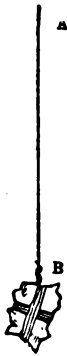
Fig. 181. A. The platinum wire. B. The fragment of "bort" or refuse diamond, considerably enlarged.
