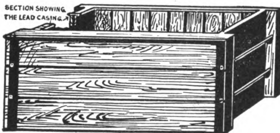
Fig. 226a. Solution vat, made of wood, showing a casing, or lining, of lead between the two surfaces, as described above.
