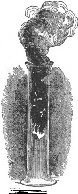
Fig. 169. Remarkable deposition of carbon during the combustion of one volume of olefiant gas with two of chlorine.
