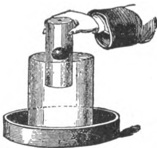
Fig. 18. The orange has entered the glass vessel, and the air having passed from the orifice, no water overflows.
