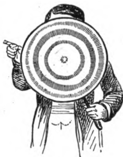
Fig. 391. The spectator is supposed to be looking towards a mirror through the slits. It is supported by a handle through the centre, round which it is twirled by the hand.
