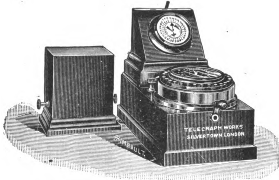
Fig. 258. Wheatstone's A. B. C. Instruments, one set consisting of indicator, communicator and bell.
