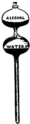
Fig. 480. Glass bulbs and tube to show the contraction in bulk of a mixture of alcohol and water.
