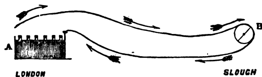
Fig. 252. A. The battery. B. The instrument. The arrows show the passage of the electricity to the single needle telegraph instrument by one wire, and the return current by the other.
