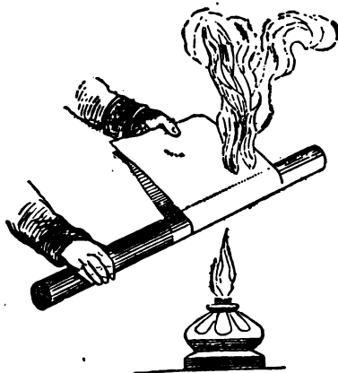
Fig. 458. Cylinder, half brass and half wood. The paper strained over the wood is taking fire. The other extremity, shaded, is the brass portion.
