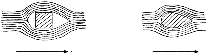
FIG. 58—Stream line construction.
