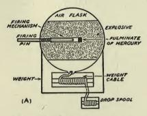
FIG. 48. A SIMPLE CONTACT MINE.
