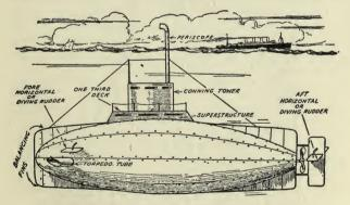
FIG. 9. THE HOLLAND SUBMARINE BOAT.
