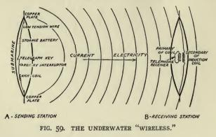
is a fairly good conductor of electricity, is made to carry an ordinary battery current between the sending and the receiving stations.
