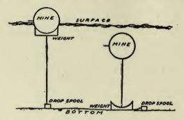
FIG. 49. HOW THE MINE ADJUSTS ITSELF.
