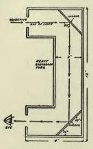
FIG. 51. HOW TO MAKE A SIMPLE MIRROR PERISCOPE.
