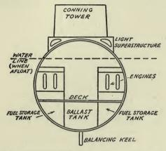
FIG. 23. CROSS-SECTION OF COAST-GOING SUBMARINE.
