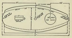
FIG. 18. HOW THE DECK IS MADE.
