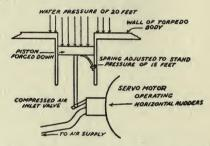
FIG. 40. HOW THE WATER PRESSURE CONTROL ACTS.
