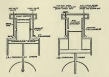
FIG. 32. A TWO-CYCLE DIESEL ENGINE.
