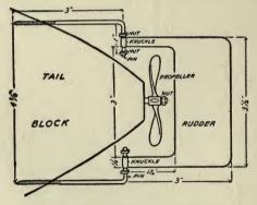
FIG. 22. THE RUDDER AND PROPELLER.
