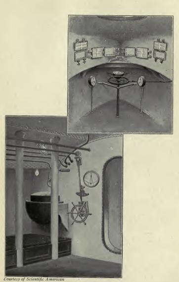
THE CONNING TOWER (UPPER) AND NAVIGATING COMPARTMEN'I' (LOWER) CONTROLS OF A MODERN SUBMARINE
