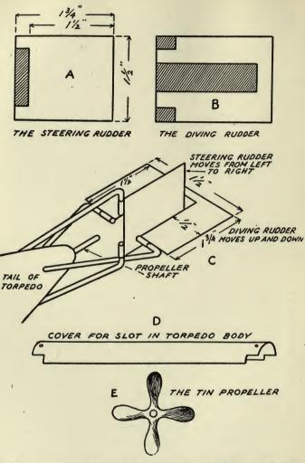
FIG. 37. A, B, C, THE STEERING AND DIVING RUDDERS. D, E, THE COVER AND PPROPELLER.
