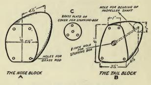
FIG. 12. THE NOSE AND TAIL BLOCKS.
