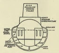
FIG. 24. CROSS-SECTION OF OCEAN-GOING SUBMARINE.
