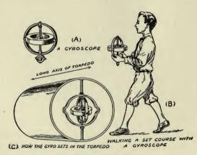
FIG. 39. THE GYROSCOPE.
