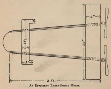
from the propellers, making the plane serve as a cross piece to hold them firmly in position. The strands of the motor should preferably be carried above the plane. This plan does away with the rear stick of the motor base, thus saving this weight. Adjust the parts very carefully, that the frame will be rigid enough to stand the strain of the motor.
