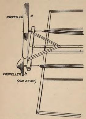
Showing an Excellent way of Fastening the Propellers to the Frame-Work.
