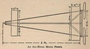
structed of metal tubing, but the cross piece supporting the propellers and the braces as well are of the same material. The new metal, "magnalium," has been used successfully for this purpose. It is a trifle heavier than aluminum, but much stronger, and almost
