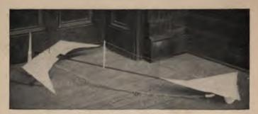
A test of high aspect ratio planes
