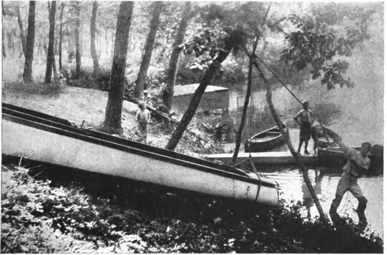
PUTTING THE "ADELAIDE" OVERBOARD ALONG WITH A PAIR OF SHEARS
