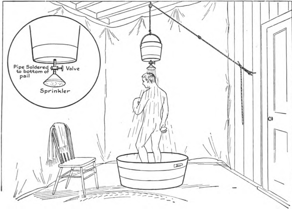
A Shower Bath That Costs Less Than One Dollar to Make
