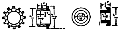
Armature-Ring Core, Its Hub and the Construction of the Commutator and Its Insulation
