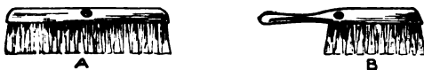
A Discarded Push Broom Shaped to Form a Brush for the Bench or Counter
