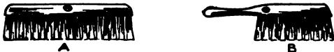
A Discarded Push Broom Shaped to Form a Brush for the Bench or Counter
