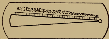
Fig. 8. Pocket Screw and Wire Gauge.
