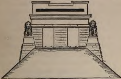
FIG. 98 b .—Abutment Tower.
