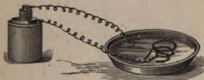
FIG. 145.—Battery and cell for electro-plating.
