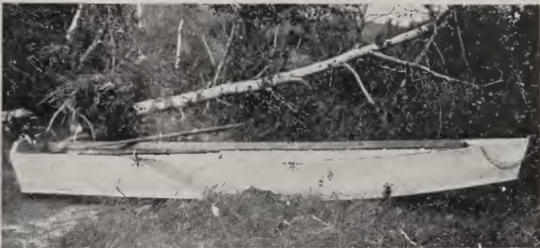
FIG. 505.—THE FLAT-BOTTOMED SHARPIE IS WELL ADAPTED TO THE OUTBOARD MOTOR.
