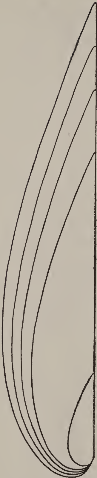
FIG. 236.—Full-Size Wing Sections for a Model of the Ford Tri-Motor. (See Plan in Fig. 233.)
