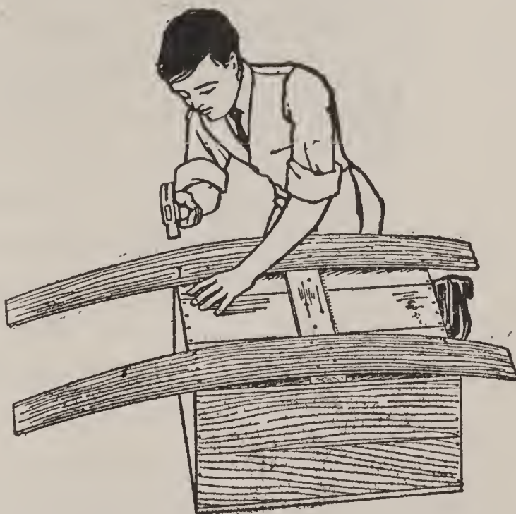
FIG. 297.—Nail Stave Runners to Box.
