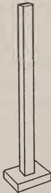
FIG. 461.— Make Tamper Like This for Tamping Concrete.
