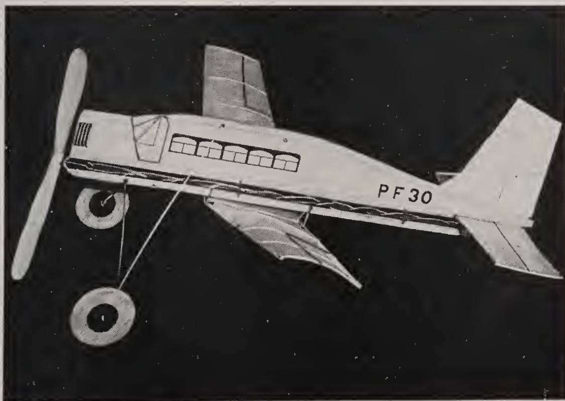
FIG. 183.—ANOTHER PROFILE FUSELAGE MODEL AIRPLANE, THE P F 30. THIS LARGER BABY, WITH LOW WING, BARELY TIPS THE SCALES AT ONE-QUARTER OUNCE.
