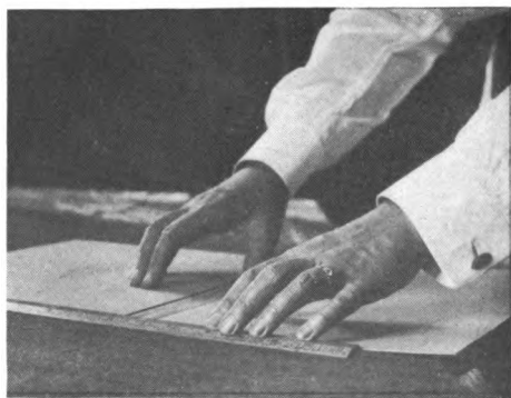
PLATE XXXVII. Pasting the newsboard to the vellum back.
