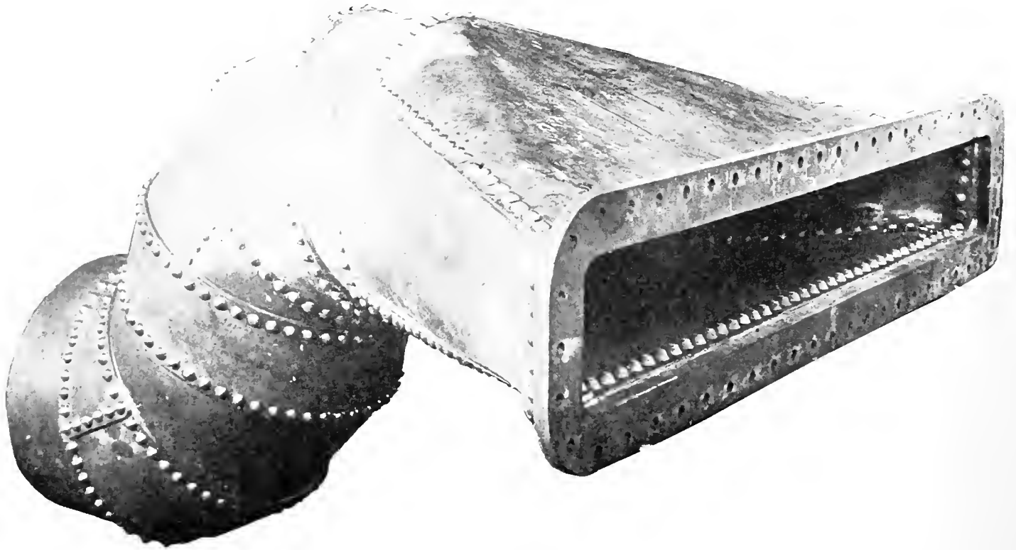
SPECIAL ELBOW USED AS AN EXHAUST CONNECTION FROM A TURBINE CASING TO A CONDENSER, CONSTRUCTED OF 7/16 -INCH PLATE AND RIVETED TO CAST-IRON FITTINGS AT EACH END.
