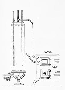
Fig. 1.-Side and Top Connections.
