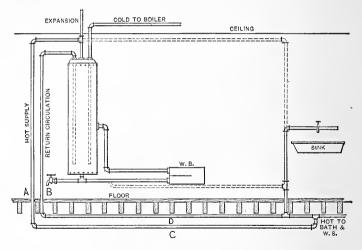
Arrangement of Circulating Pipe.
