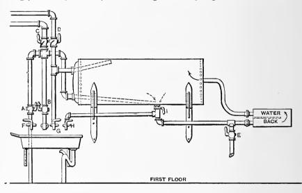
Fig. 1.-Method of Setting Boiler.
