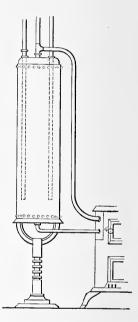
Fig. 2.-Bottom and Top Connections.
