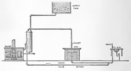
Fig. 1-The Original Arrangement of Pipes.
