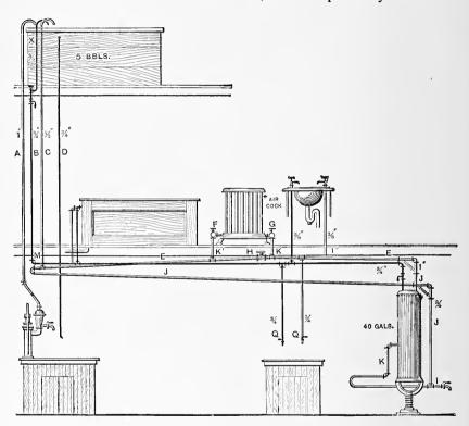
A Plan for Heating Bathroom.
