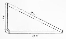
Fig. 1.-Two Ways of Running Pipe.
