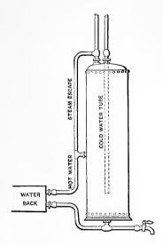
Fig. 1.-Remedy for Noisy Range Boiler.
