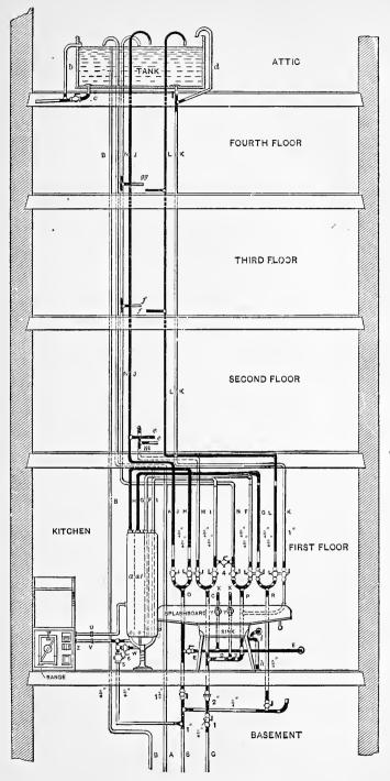
Double Boiler System of Plumbing.
