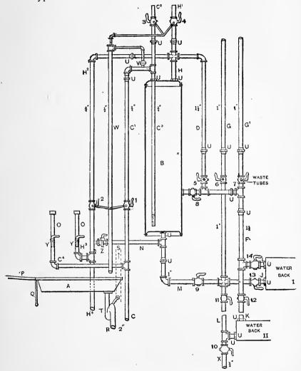
Fig. 4.-Range Boiler and Connections.
