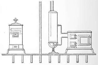
Boiler Connected with Two Stoves.
