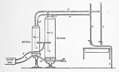
Fig. 1.-Faulty Way of Connecting.
