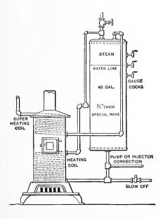
Fig. 2.-Ryan's Steam Apparatus.
