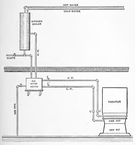
Water Heating by Gas or Furnace.
