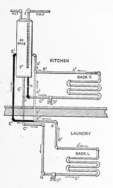
Fig 2.-Proposed Change in Pipe Connections.
