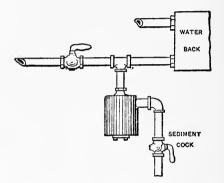
Fig. 3.-Sediment Chamber.
