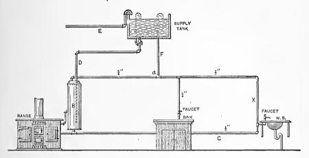
Fig. 3.-Showing Proper Arrangement of Pipes.
