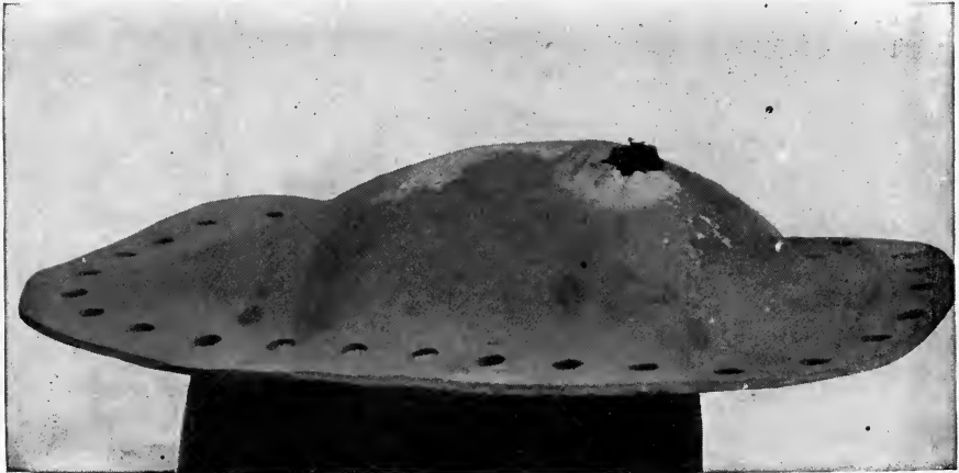
FIG. 28.—A Bagged Plate.
