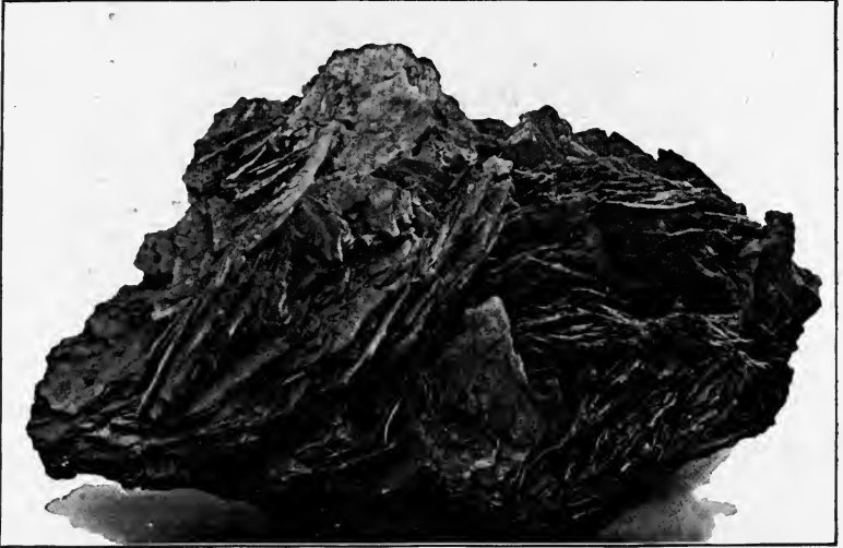
EXHIBIT NO. 1. SCALE BETWEEN SHELL AND TUBES. (C. S. Garrett & Son Co., Buck Run, Pa.)
