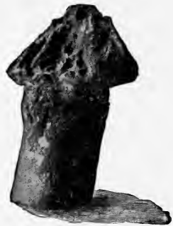
FIG. 9.—A Corroded Rivet.
