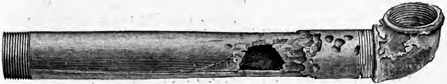
FIG. 25.—Corroded Brass Pipe from the Interior of a Boiler.
