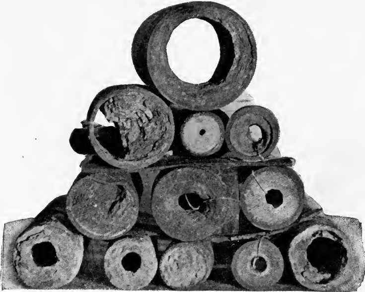
FIG. 6.—Accumulation of Scale in Flue Ends.
