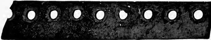
FIG. 22.—A Pitted Plate—Inner Lap.
