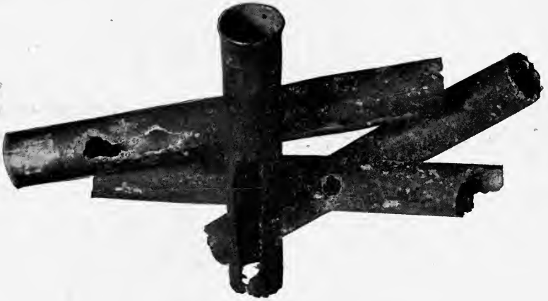
FIG. 24.—Effect of Electrolysis upon Brass Tubes.
