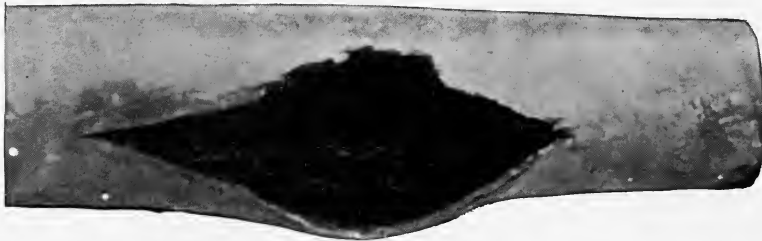
FIG. 22a.—Ruptured Blow-off Pipe.
