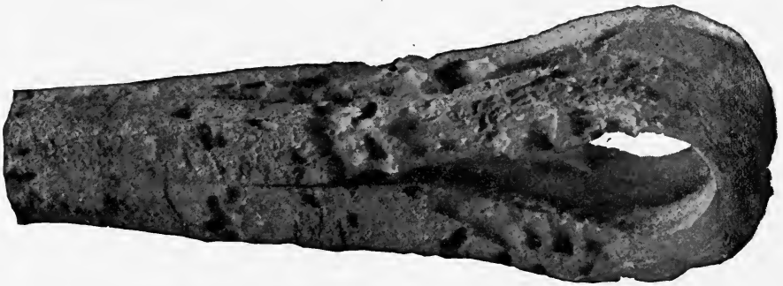
FIG. 8.—A Corroded Brace.
