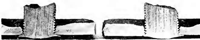
Fig. 2.—Result of Weaving Action on Inner Bolt Connections
