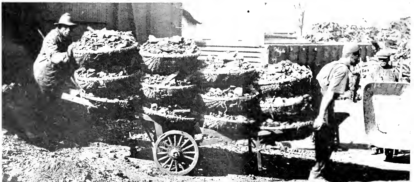
Fig. 3.—Sixteen Thousand Bushels Like These are Used at the Plant Each Week in Making Charcoal Iron Boiler Tubes
