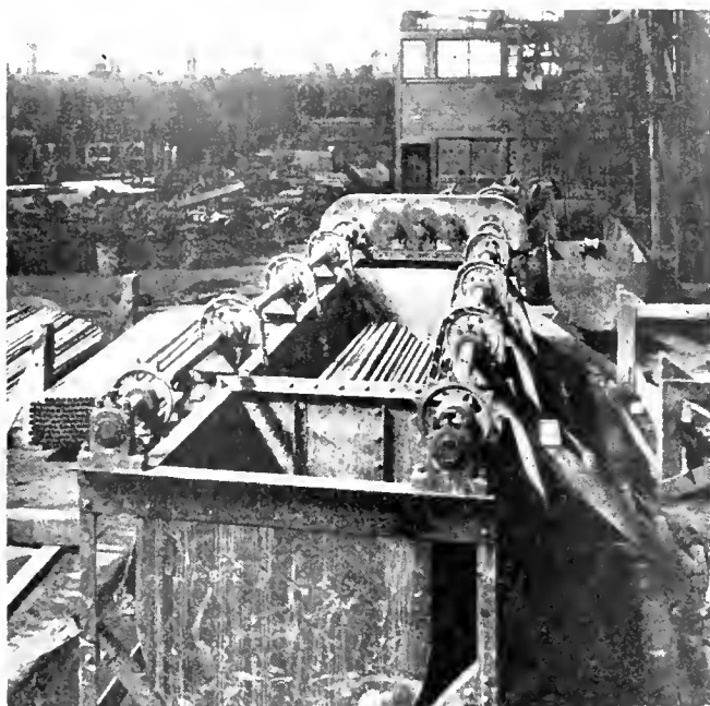
Small Tubes Being Cleaned in Wet Rattler
