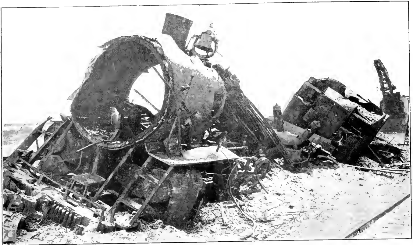
Fig. 1.—Results of a Low Water Explosion in Which the Water was Ten Inches Below the Top of the Crown Sheet at the Time of the Accident
