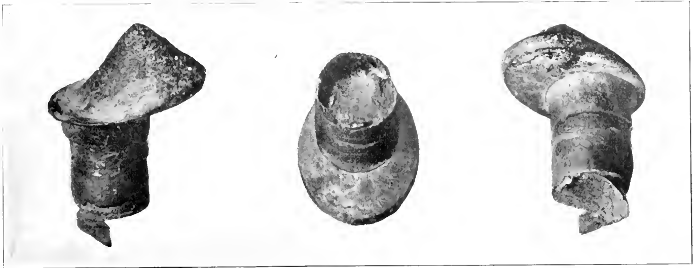
Three Views of a Seriously Defective Rivet
