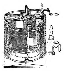
Fig. 43.—'' AUTOMATIC '' FOUR=COMB REVERSIBLE EXTRACTOR.
