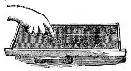
Fig. 40.—SPUR WIRE EMBEDDER IN USE.
