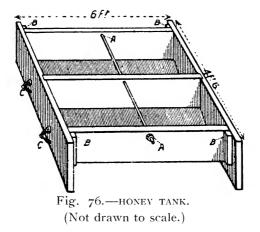
For an apiary of, say, two hundred colonies, two such tanks as the double tank illustrated would in most cases answer the purpose. There is a great advantage in dividing the tanks into compartments, so that the honey from each day's extracting may be left undisturbed until it has matured and is ready to run into tins. It is unwise to run two or three days' extracting into the same tank, as the frequent disturbance is against the honey maturing properly.
