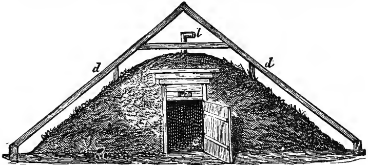
Fig. 138. (From L'Apicoltore, of Milan.) BEE CLAMP FOR WINTERING. l , air draft. d , roof.
