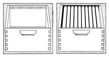
FIG. 6.—The hivebody is like an FIG. 7.—Hivebody with frames in empty box. place.
