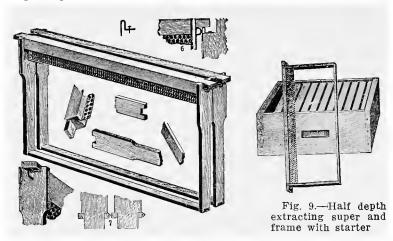
Fig. 8.—Standard Langstrothe frame with starters in place
