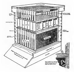
Fig. 2.—A modern hive complete. Cut away to show arrangement of brood chamber and super arrangement
