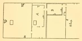
The room is ceiled with matched boards and a space of 18 inches is left from the partition to the wall. The cellar bottom is all cemented; size of this room is 16 by 9 feet and  $6\frac{1}{2}$  feet high. The cellar windows on the north and south side are loosely packed with straw so that air is admitted freely.
