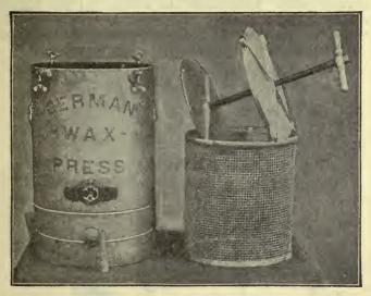
Fig 21.-Root-German Steam Wax-press. (After A. I. Root Co.)
