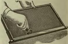
Fig. 5.—Foundation roller for fastening in frames. (After A. I. Root Co.)
