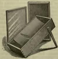
Fig. 14.—Doolittle solar wax extractor.
