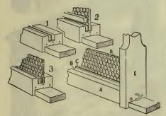
Fig. 4.—Method of inserting foundation into Hoff-man frames. (After A. I. Root Co.)
