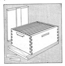
Fig. 52-"Dovetailed" or Lock-Cornered Hive
