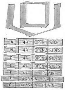
Fig. 102—Sections of Different Widths and Openings.
