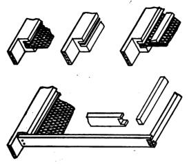
Fig. 58-Insertion of Foundation in Frame.
