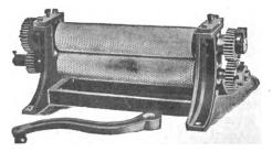
Fig. 86-Comb Foundation Mill.
