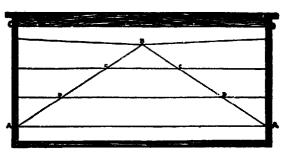
Fig. 5—This plan has been used very largely in California. It was there the author saw that brood in the combs wired this way would go clear to the top bar.
