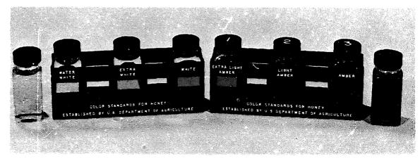
U. S. Department of Agriculture honey color classifier or comparator used to determine the color classification and turbidity of a given honey sample. It has to a large extent replaced the Pfund grader in this use.
