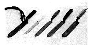
Uncapping knives. Steam heated on the left, electrically heated on the right. The three in the center are heated in a hot water bath.
