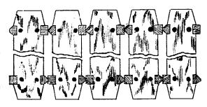
Drawing showing how the sharp edge of the end bar touches the square edge cutting the propolis accumulations.
