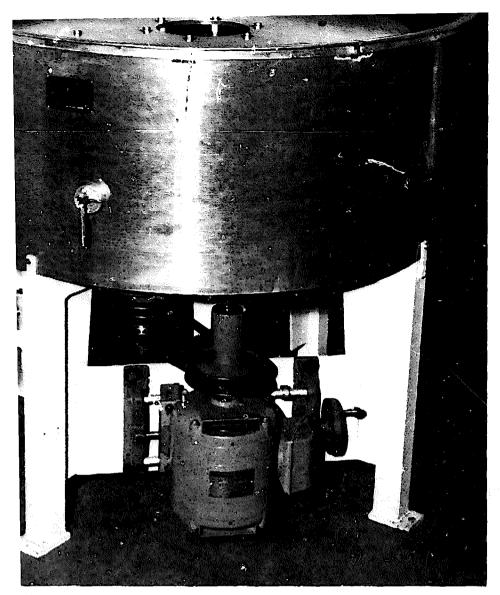
handle a large volume of cappings and honey. Separation is by contribugal arce when the inside drum is spinning — Photo by J. Bailey.
