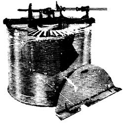
Fig. 5—Root Simplicity radial extractor that does not require reversing. The real is surrounded with perforated metal to catch particles of comb that would clog the honey pump.
