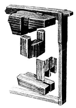
This method of interlocking of frame parts insures strength.
