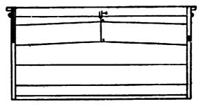
Fig. 6—This will prevent sagging, but is too complicated and does not permit of electrical imbedding.
