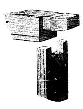
Improved Root-Hoffman end-spaced frame. Some apiarists prefer top bars just enough shorter to leave a bee space between the ends of the frames and the hive. The ends will thus be free of bee glue. End-spacing staples keep the frames from going too far endwise.
