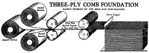
now Three-ply is made: As its name implies, this famous foundation is made of three sheets of beeswax rolled together into one to form a tough sag resistant foundation.
