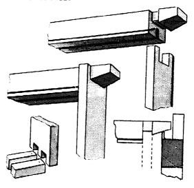
Detail showing the lock corner construction and how the projection rests on the metal support in the upper end of the hive.
