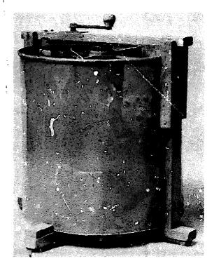
The original extractor made and used during his life by Moses Quinby. Note the heavy spur gears, the oak cross bar, the oak framework underneath, forming a support for the lower bearing.
