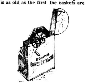
Fig. 2—An early extractor in which the combs are whirled vertically. Reproduced from Gleanings in Bee Culture for November 1, 1893.
