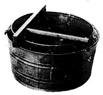
Uncapping can. This separates the free honey from the cappings as they fall from the uncapping knife. The cappings are held in the perforated basket while the free honey drains into the tub below.
