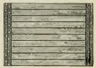
FIG. 75.-Grooved Board for Cutting Starters.
